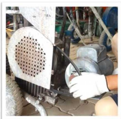
③ Slightly unload the motor, and untie the belt from the motor.
